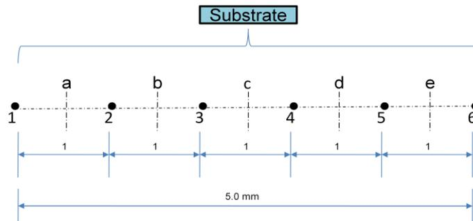
**Figure 3 One Dimensional Grid Set Up for an Uncoated Substrate**
