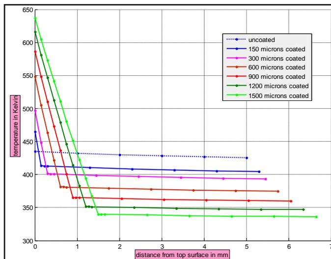
**Figure 6: Effect of Top Coat Thickness on Temperature Distribution along Thickness after 5s of Thermal Loading**
