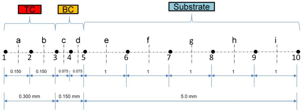
**Figure 2: One dimensional Grid Set Up for a TBC Coated Substrate**
