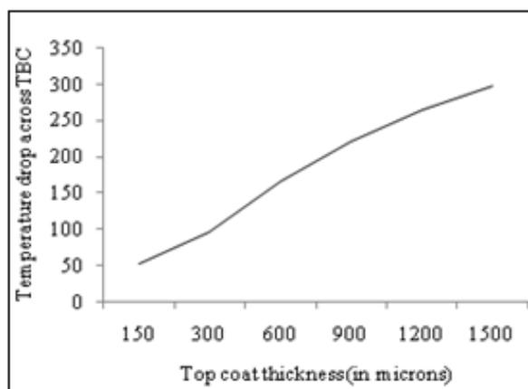
**Figure 8: Temperature Drop in Y-PSZ/NiCrAlY TBC Set Up after 5s of Thermal Loading at Different Y-PSZ Coating Thicknesses**
