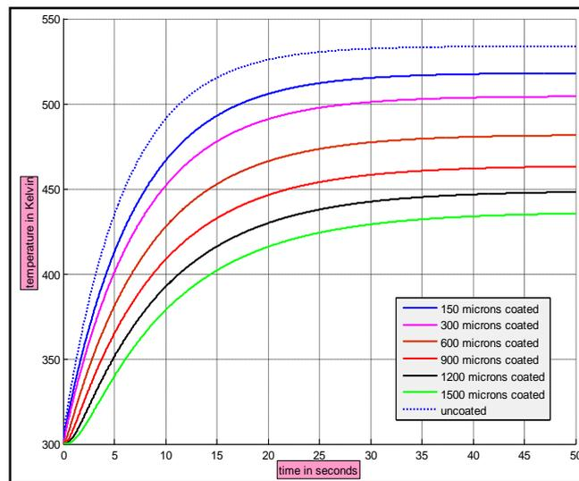
**Figure 4: Effect of Top Coat 8Y-PSZ Layer Thickness on Top Substrate Transient Temperature**
