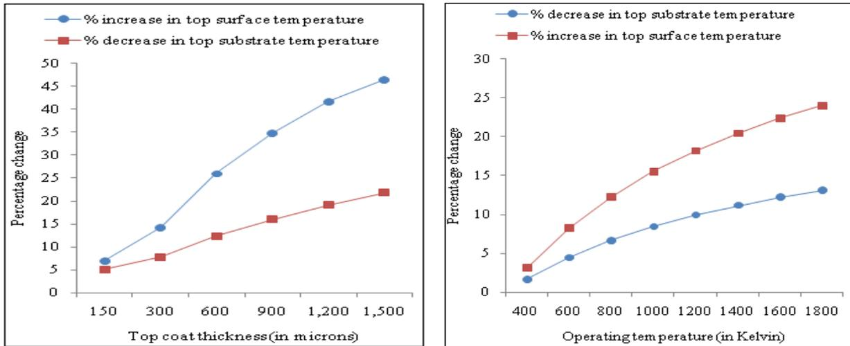
**Figure 7: Percentage Changes in Top Surface Temperature and Top Substrate Temperature after 5s of Thermal Loading at Different Coating Thicknesses (left) and Different Operating Temperatures (Right)**
