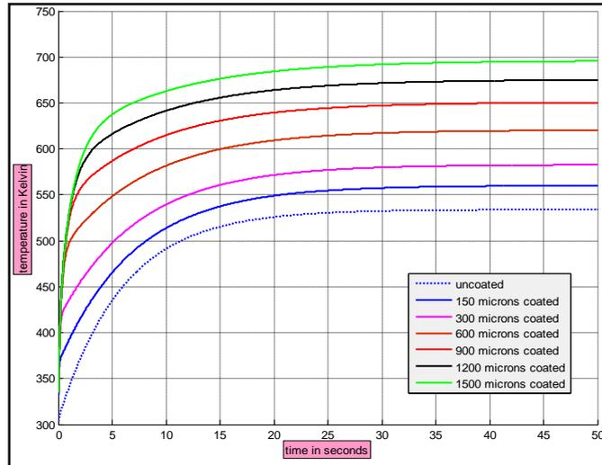
**Figure 5: Effect of Top Coat 8Y-PSZ Layer Thickness on Top Surface Transient Temperature**
